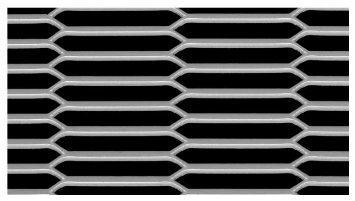
LW Pitch:133.33mmStrand Width:3.00mmSW Pitch:12.90mmThickness:3.00mmWeight:10.50 kg / m2 (Black Weight)Open Area:53%
